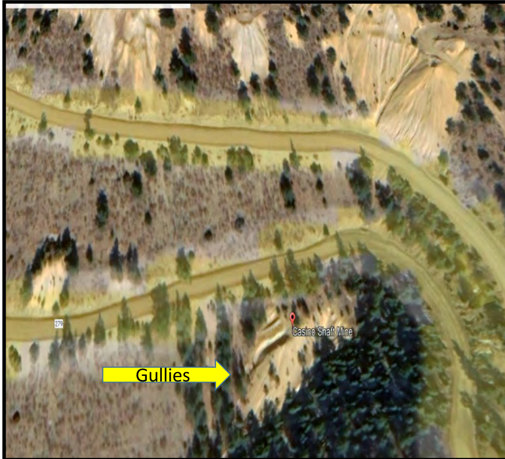
Casino Mine Pre-Reclamation. Deeply incised Gullies and No Vegetative Cover (2019)—Image From Google Earth
